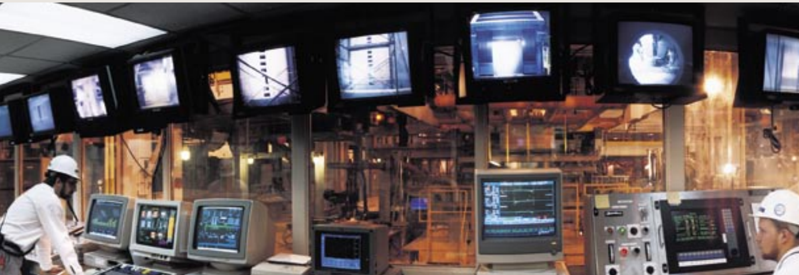
Workers at PRO-TEC's process pulpit monitor the continuous galvanizing process with the aid of computers and video imagery.
