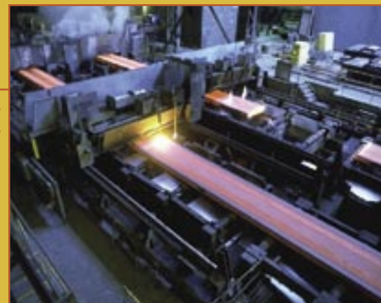
Torch-cutters cut slabs as they are turned out at Mittal Steel USA.
